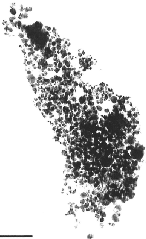
Figure 4. Transmission electron micrograph of the SPMP synthesized in the cross-linked starch by using potassium nitrate as an oxidant for iron
